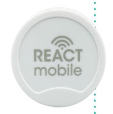
The React 2.0 Beacon device is a discreet, easy to conceal device that allows our safety platform to deliver precise room level location accuracy indoors in multi-story buildings.
